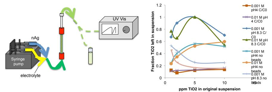
Batch and column studies allow investigation of TiO<sub>2</sub> attachment at low concentrations (~100 ppb).
